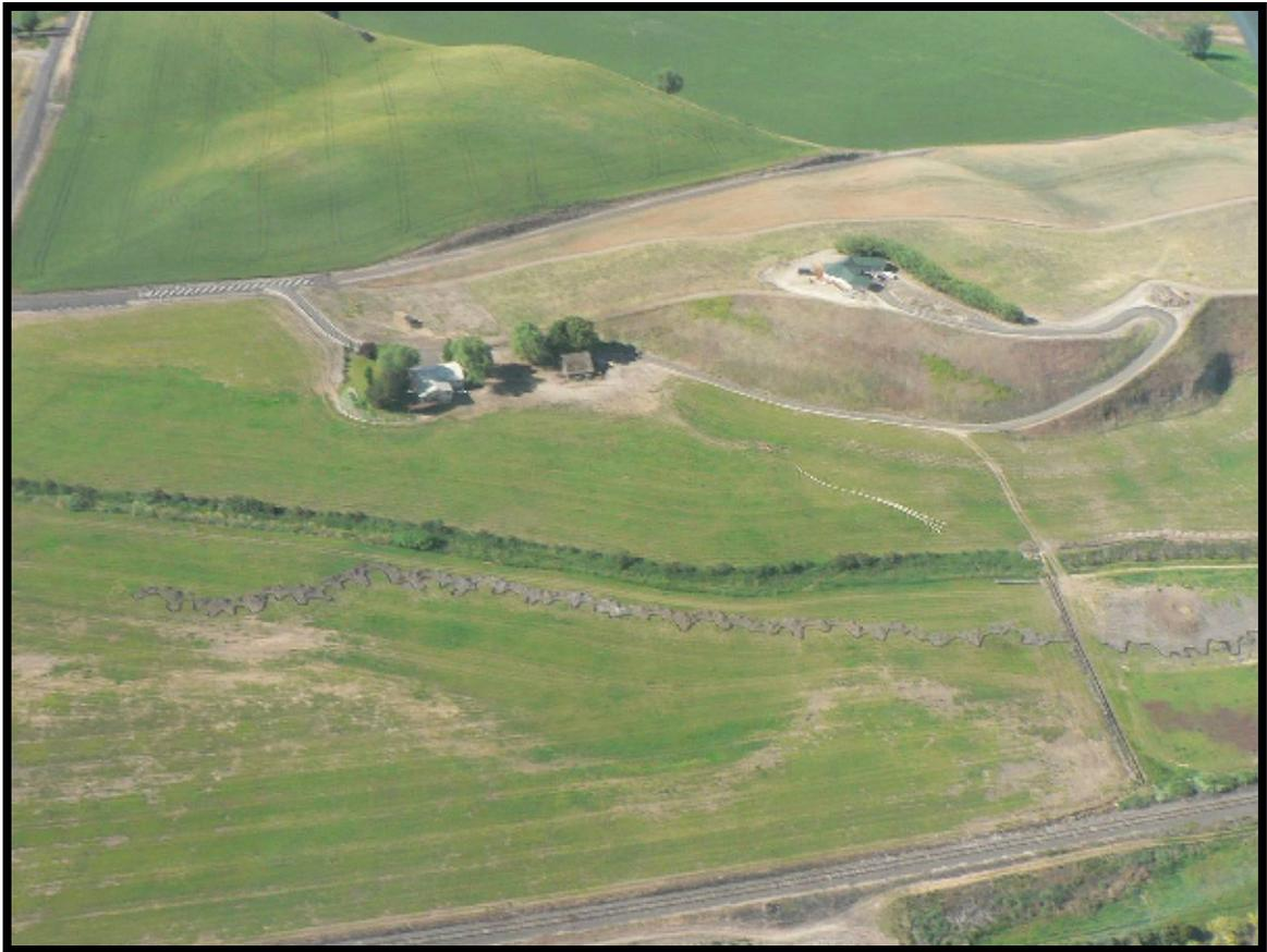
***The new meandering channel of Doan Creek is shown just below the irrigation channel (in dark green). The new meander pattern was designed by WDFW staff and increased the stream length from 1900 ft. to 4100 ft.***
