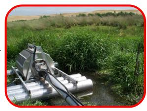
gation pump intakes while protecting landowners from regulatory penalties from non-compliant screening. Screen capacities range from 15 gpm to 10 cfs (4500 gpm).
