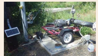
New meter for irrigation diversion with solar power. Renewable energy holds many possibilities.
