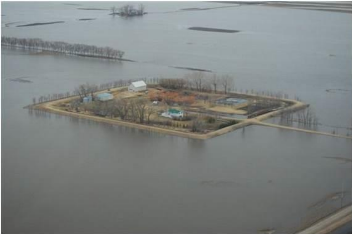
Figure 21. Ring dike protecting property in floodplain in areas where levees failed
