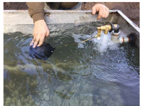
Water trough allows cows to drink and protects water quality in Dry Creek. Photo by Joanna Cowles Cleveland
