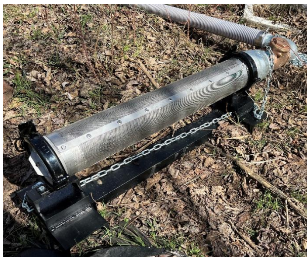
Figure 2: Surface diversion fish screen replaced with VSP cost-share funds
