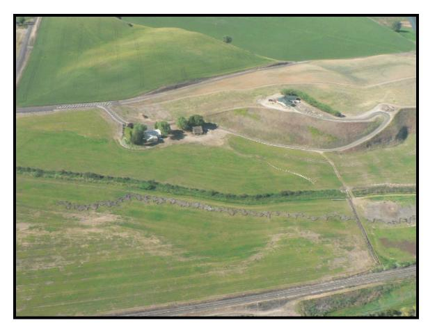
The new meandering channel of Doan Creek is shown just below the irrigation channel (in dark green). The new meander pattern was designed by WDFW staff and increased the stream length from 1900 ft. to 4100 ft.
